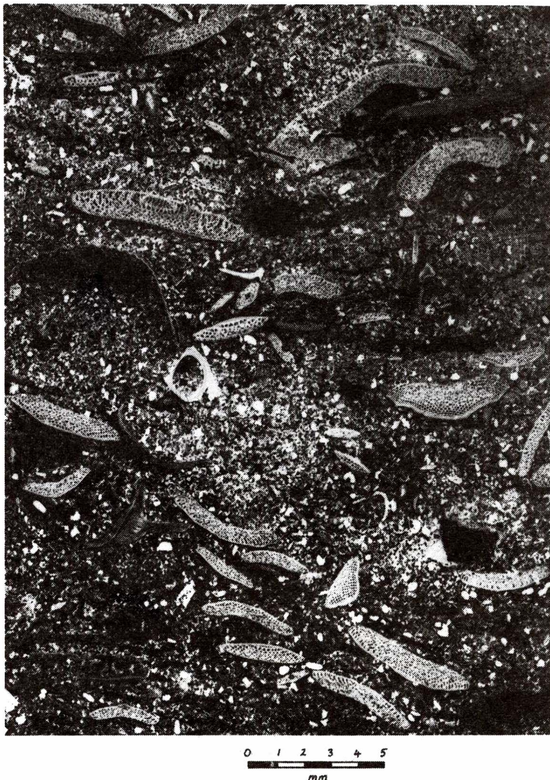
Plate 1. Orbitolina biosparite. Allochems, including many tests of Orbitolina , and other grains are cemented mainly by sparite, but micrite is patchily present. Negative print from a thin section.
