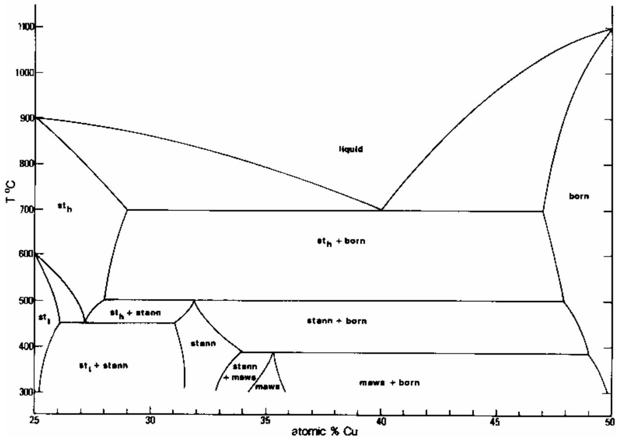
Figure 3. Hypothetical phase relationships in the pseudobinary system stannite-bornite, for zinc-bearing stannite and stannoidite. Symbols: st<sub>h</sub> = high stannite polymorph; st<sub>l</sub> = low stannite polymorph; stann = stannoidite; maws = mawsonite; born = bornite.
