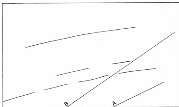
Figure 3(b) Interpretation of (a). A = thrust plane, B= reflected refractor arising from a fault off-section. Other lines are interpreted as bedding within the thrust slice.
