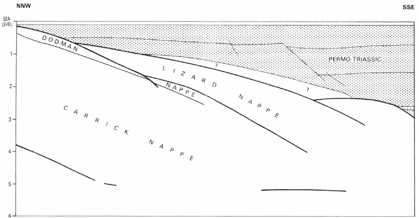
Figure 1(b) Interpretation of (a) showing the strong reflectors in the basement interpreted as thrust planes. Figures on the left side are two-way time in sees. Length of profile is 28km.
