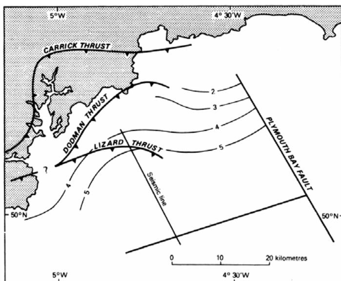
Figure 2. Two-way reflection time map of the prominent reflector in Devonian basement south of Cornwall identified as the Carrick Thrust; isochrons in seconds. Seismic events sub-cropping the Permo-Triassic sediments are shown, which are interpreted as the Dodman and Lizard Thrusts. The position of the Carrick Thrust is inferred from land observations. The line of the seismic section of Figure 1 is shown.
