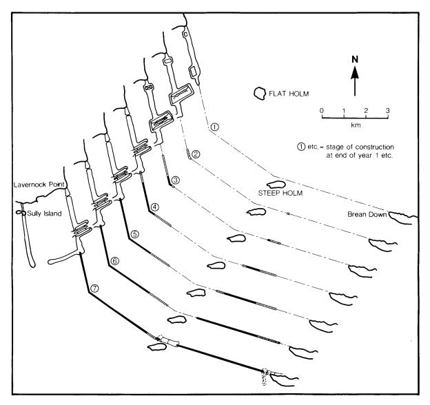
Figure 3. Plan view of seven yearly stages in construction of a Cardiff-Weston Barrage using prefabricated caisson construction (courtesy of STPG).
