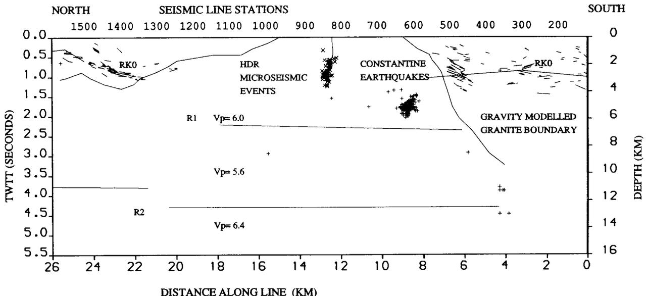
Figure 3. Combined geophysical data on line HDR/002 showing immigrated reflection
