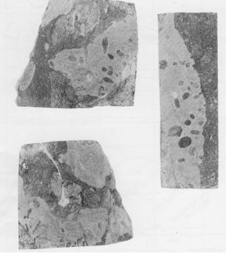
Figure 1: Photographic montage of three blocks of the basal conglomerate from the working quarry on Hamdon Hill. The long vertically arranged block is 12 cm long. The other blocks are the same scale.
