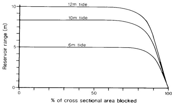
Figure 4. Graph showing the influence of works upon the tidal range. Tidal range does not become noticeably modified until after more than 80% of the cross-section is blocked. By this stage a crossing will be completed.
