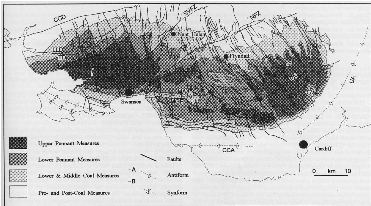
Figure 1. Map of the South Wales Coalfield (After BGS 1:50 000 range geological map) showing the main structural elements and the location of Nant Helen and Ffyndaff OCCS. CCD=Carreg Cennen Distrubance, LLD=Llanon Distrubance, TD=Trimsaron Distrubance, SVFZ=Swansea Valley Fault Zone, NFZ=Neath Fault Zone, MA=Maesteg Anticline, MGF=Moel Gilau Fault, CCA=Cardiff-Cowbridge Anticline, CS=Caerphilly Syncline, PA=Pontypridd Anticline, GS=Gelligaer Syncline and UA=Usk Anticline.
