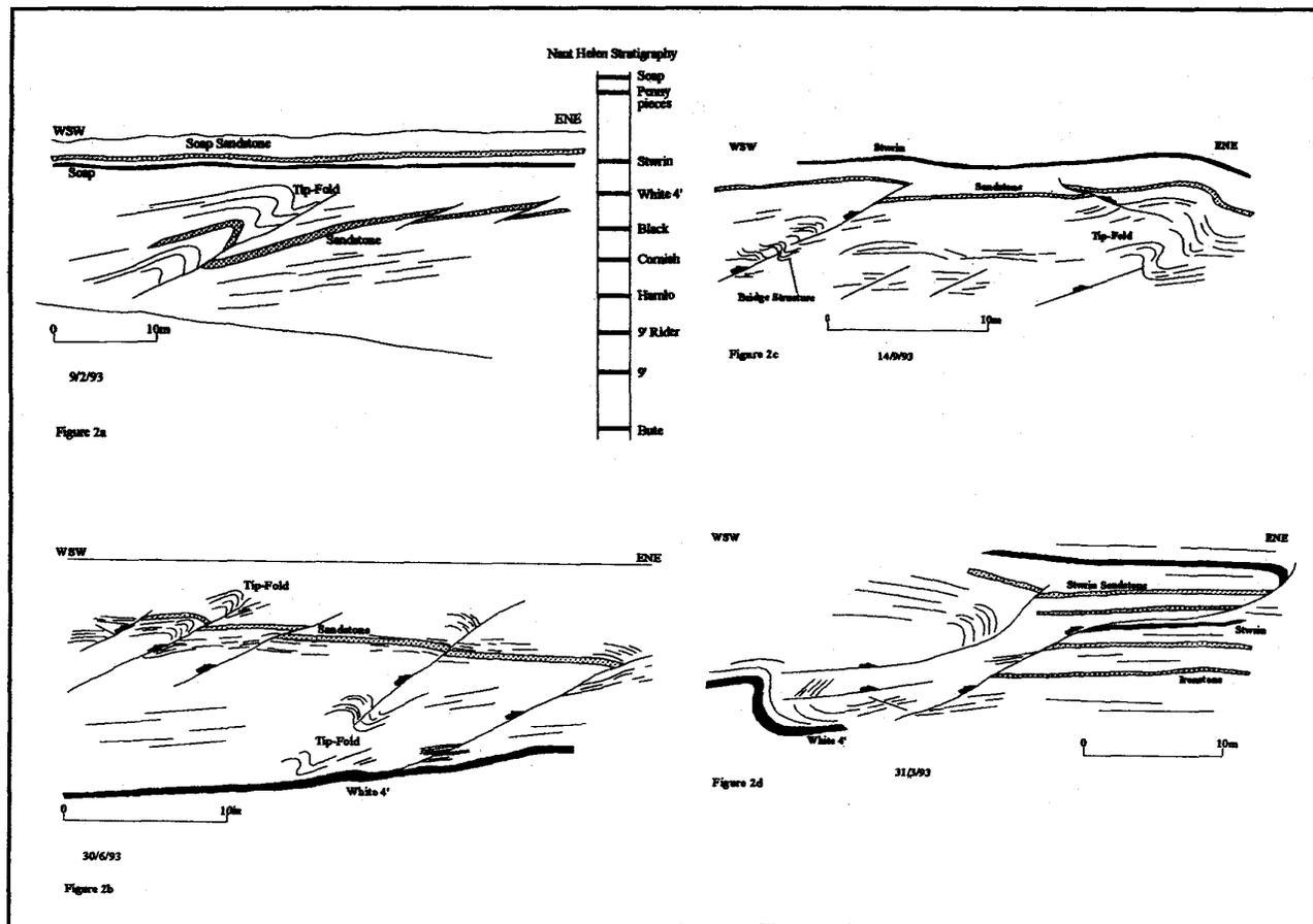
Figure 2a. West south-west to east-south-east face section of the sequence between the Stwrin and Soap seams at Nant Helen OCCS showing isolated thrusts cutting a thin sandstone and mudrocks above and below. The western most thrust shows tight folds in the hangingwall interpreted as tip-folds cut by later thrust propagation.
