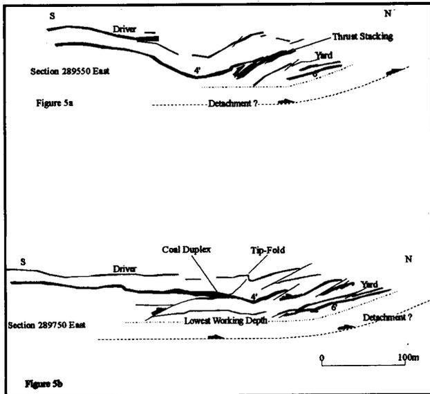
Figure 5a. Extraction section 289550E from Dunraven, showing an asymmetrical syncline in coal measures with thrust stacking concentrated on the steeper, northern limb.
