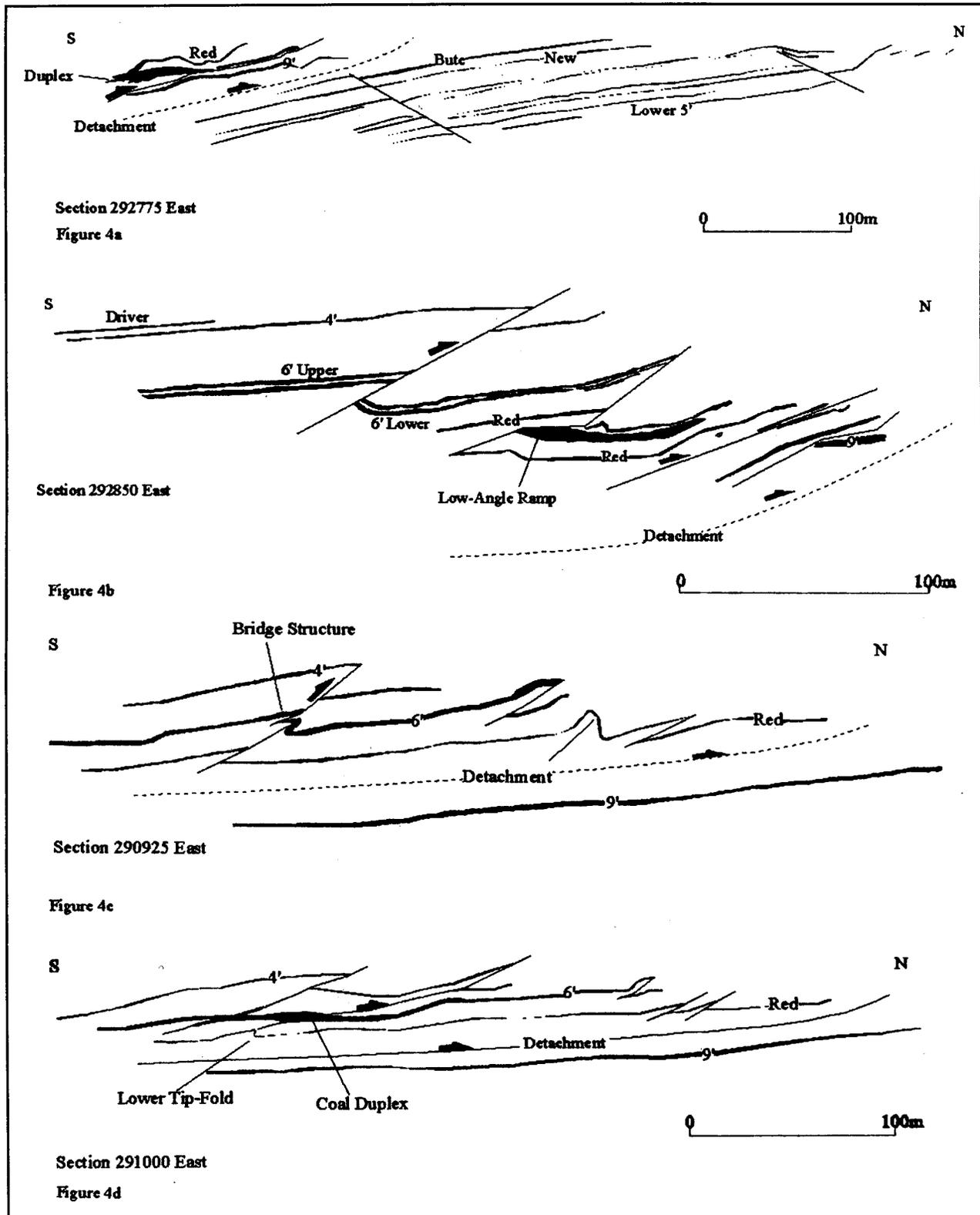
Figure 4a. Extraction section 292775E from Ffyndaff Area B, showing thrust deformation restricted to the Nine Foot seam and above. Note the duplex in the Nine Foot seam bounded in the roof by an out-of-sequence thrust.
