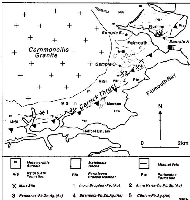
Figure 2. Gold bearing localities in the vicinity of the Carrick Thrust in the Falmouth area (trace of the thrust after Leveridge et al., 1990).
