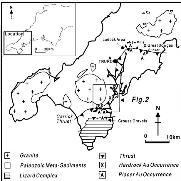
Figure 1. Hardrock and placer gold occurrences within the vicinity of the Carrick Thrust, south Cornwall (trace of the thrust after Leveridge *et al.*, 1990).
