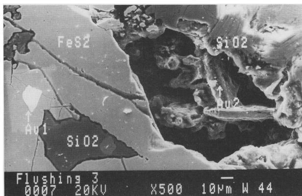
Figure 3. SEM image of gold locked in pyrite (Au 1, arrowed), and remnant gold in quartz after pyrite dissolution (Au 2, arrowed); sample A, Flushing [SW 812 338]
