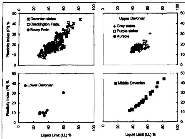
Figure 1. Plasticity of soils developed on Devonian slates in south Devon. (a) Comparison with other local high plasticity soils; the similarity with the Crackington Formation reflects their similar illite-dominated mineralogy compared with the kaolinitic Bovey Formation clays. (b) soils on Lower Devonian slates, (c) soils on Middle Devonian slates, (d) soils on Upper Devonian slates.
