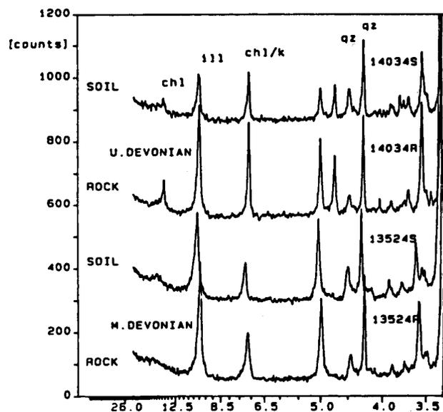
Figure 2. X-ray diffraction spectra from soil-rock pairs.
