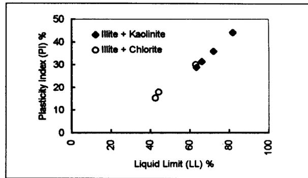
Figure 3. Clay mineralogy compared with plasticity. In each case the sample is that with the maximum plasticity from that site. Data from this study supplemented by reinterpretation of XRD data of Hunter (1997) on samples from sites where plasticity had been determined in this study.
