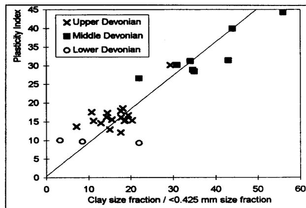
**Figure 5.** Activity of soils developed on Devonian Slates. Note the the clay size fraction is corrected for the presence of particles larger than 0.429 mm, since it is the <0.425 mm fraction on which the plasticity is determined. A line of activity — 0.9 (the activity of illite) is shown for reference.
